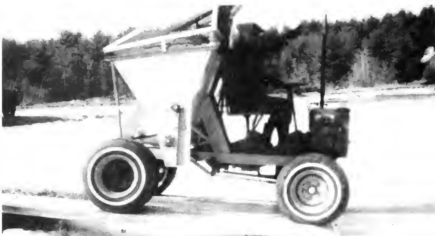
Figure 1. Sand spreader crossing a pair of aluminum bridges with 1\frac{1}{2} cu. yards of sand.
